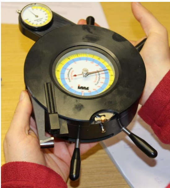
Fig. 1 Fractometer while measuring the samples: in the middle is measured the bending and compression strength and force; in the upper part the bending angle is measured. The bending angle can be used for calculation of bending stiffness.
