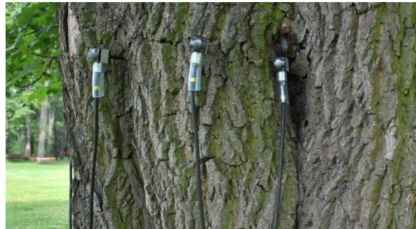
Fig. 2 Set up of sonic tomography in detail: in the case of complicated geometry is better to use more sensors. It is recommended to have one on each bulge and one in each depression.
