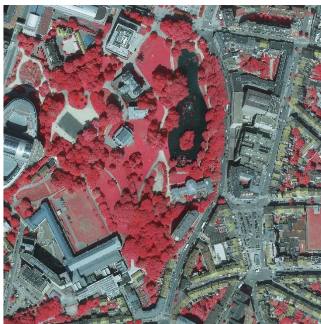
Fig. 143 example of an airborne near-IR image (the lighter red the tree, the lower its physiological condition).
