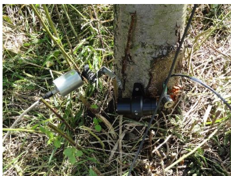
Fig. 14 Comparison of mechanical devices: left – inclinometer, middle – accelerometer (older type), right – accelerometer with high frequency (not in commercial use).
