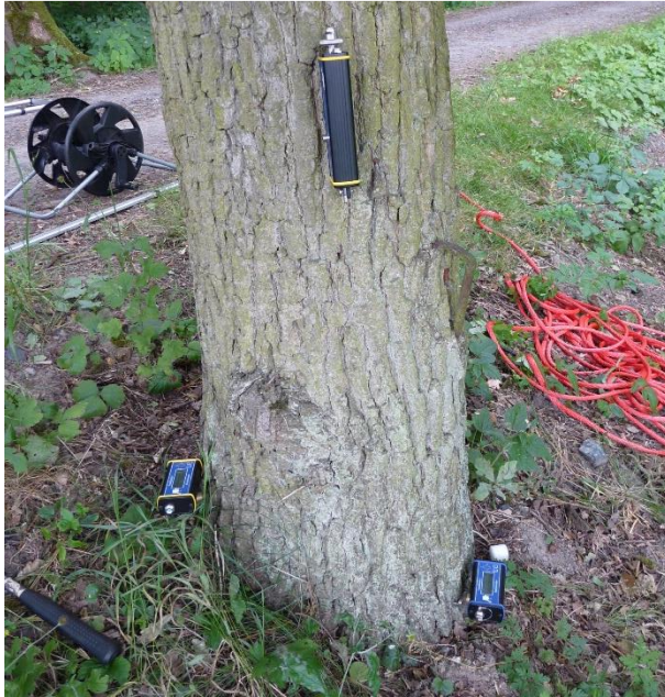
Fig. 82 Extensometer on the tension side of stem and inclinometers near the tree base.
